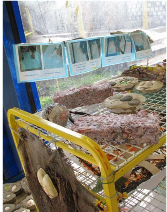
Drying the fire bricks - made from recycled kindergarten waste paper
